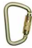
AZ017T acier zingué ouverture 25mm 113X71mm, 200 gr.
