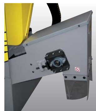
ST Scaricatore trucioli Swarf conveyor Evacuateur de copeaux
